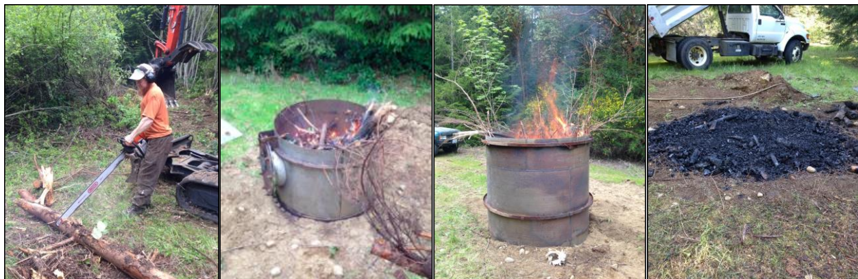
Figure 2. Use of a cylinder burner for on-site production of biochar from forest harvest residuals on the San Juan Islands, WA, USA
